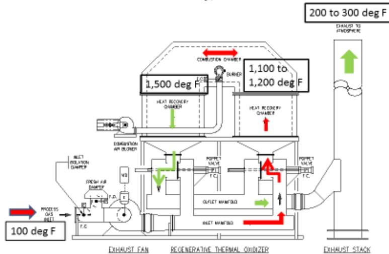
DELCORA - first application of a two-canister RTO on a MHF based system
